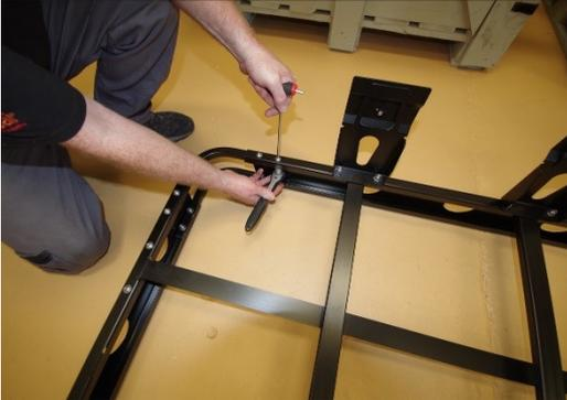
1. Fix the corner pieces to the side panels using the long bolts.
