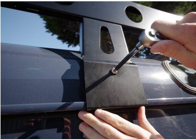
9. Lift the roof rack onto the vehicle and fasten the brackets. The brackets fit around the outside of the guttering and the legs slot inside the gutter itself. In some cases, the protective material under the brackets can obstruct the opening of the doors. If this occurs, simply remove this material or adjust the position of the door.
