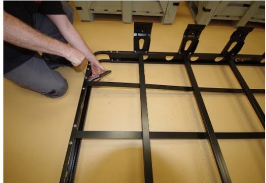
2. Assemble the crossbars running lengthways once the frame has been built.
