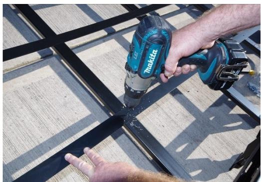
6. The crossbar intersections need to be riveted. In each intersection, drill an appropriately sized hole for the rivets you have chosen to use.
